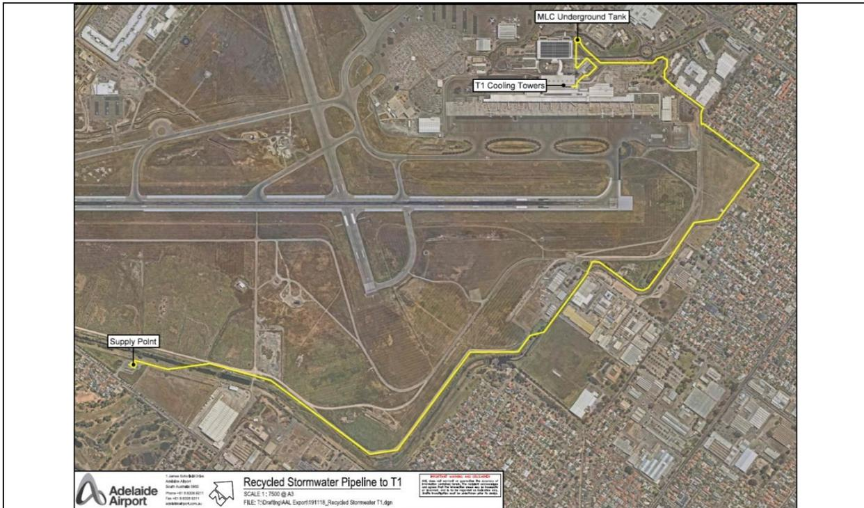
Plan showing recycled water pipeline from aquifer recharge supply point to MLC underground tank and then to T1 cooling towers
