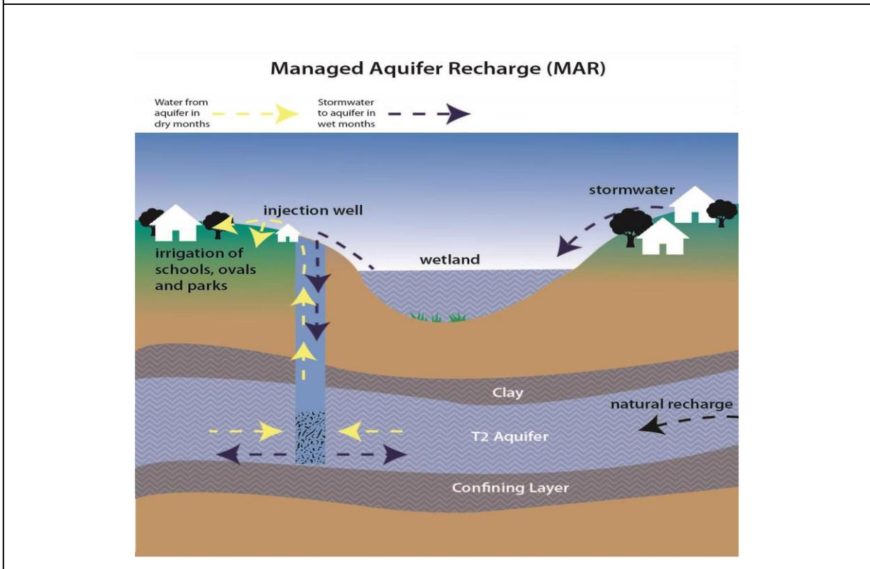
Schematic showing Managed Aquifer Recharge
